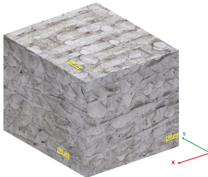
Figure 3.13. 3D representation of microstructural characteristics of SLM manufactured IN 625 in as-built state (magnification 100x)
