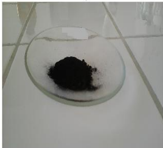
Fig. 3.38. Cathode paste calcined at 400 °C.
