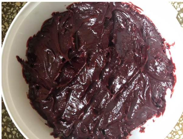
Figure 13. Grease experimentally made from used oils (variant 4)
