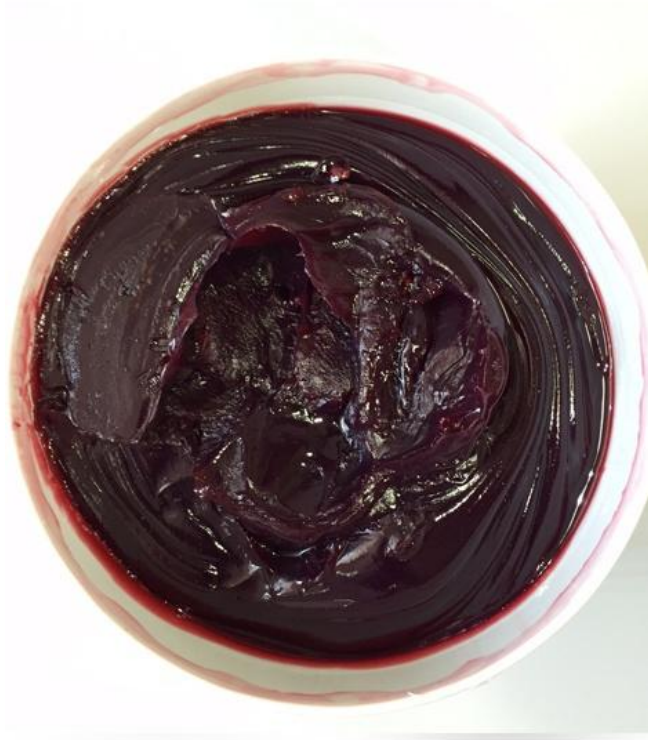
Figure 12 Experimentally made grease from waste oils (variant 1)
